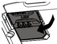
Insert the battery. The golden contacts on the battery must face towards the bottom right. Press lightly on the top end of the battery until it snaps into place.
