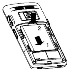
Replace the battery compartment cover back on the phone. Slide the battery compartment cover upwards until it snaps in to place.
